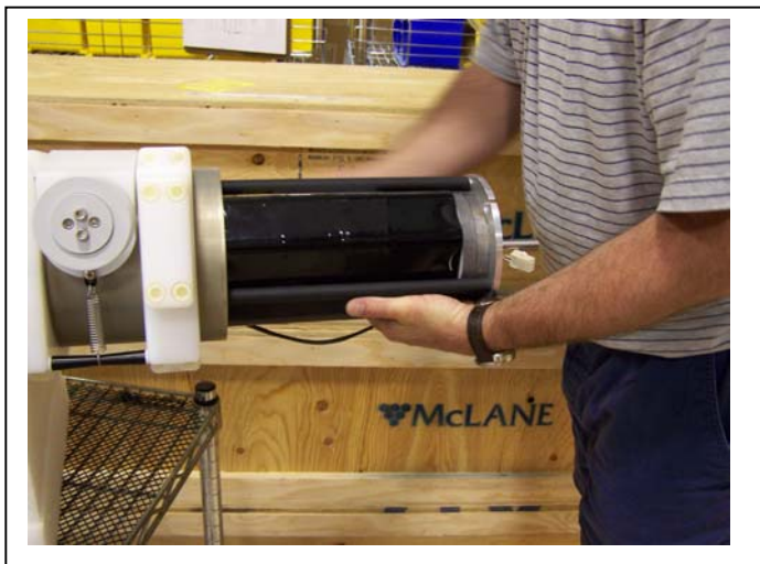
Figure 2-10: Slide in Electronics Chassis
