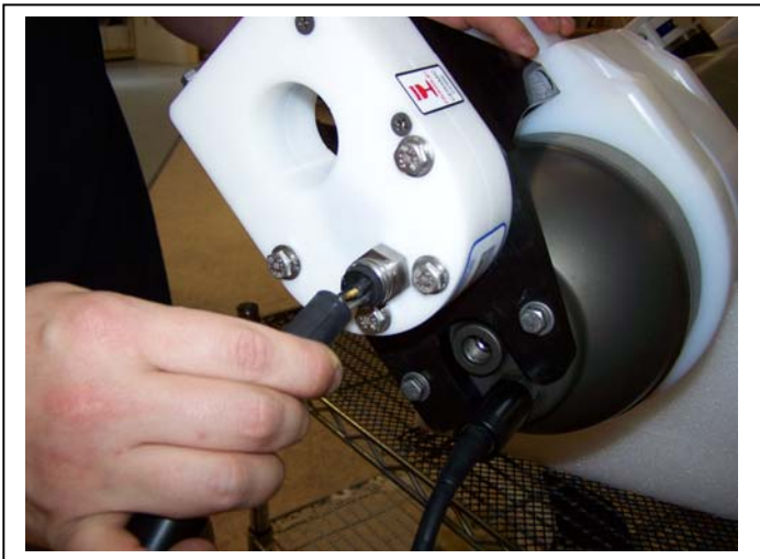
Figure 2-24: Connect UIM Cable
