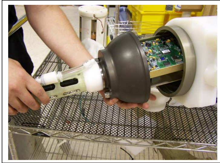
Figure 6-4: Remove the Chassis
