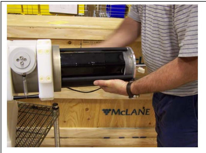
Figure F-6: Slide in Electronics Chassis
