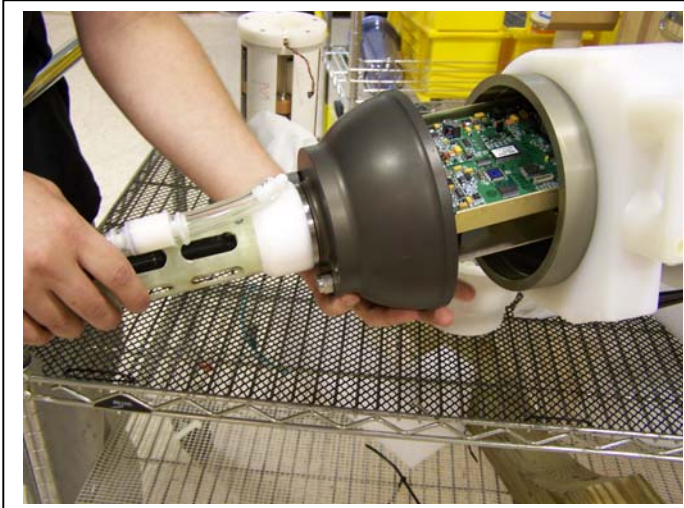
Figure 2-15: Slide in CTD Electronics
