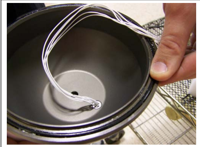
Figure 2-18: Inspect and Reseat O-Ring
