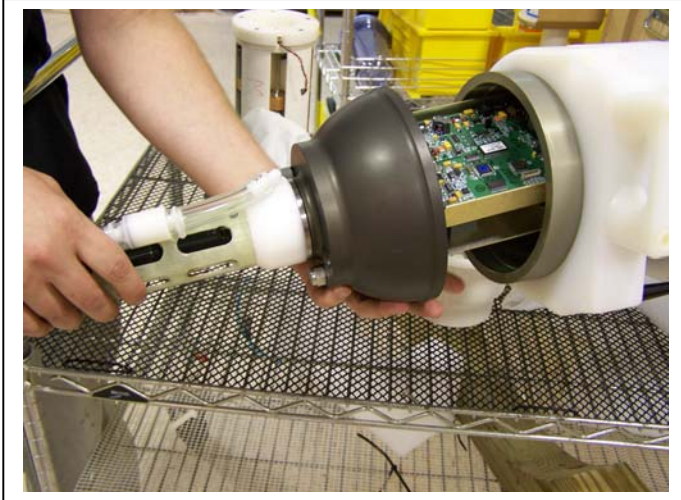
Figure F-12: Slide in Sensor Electronics
