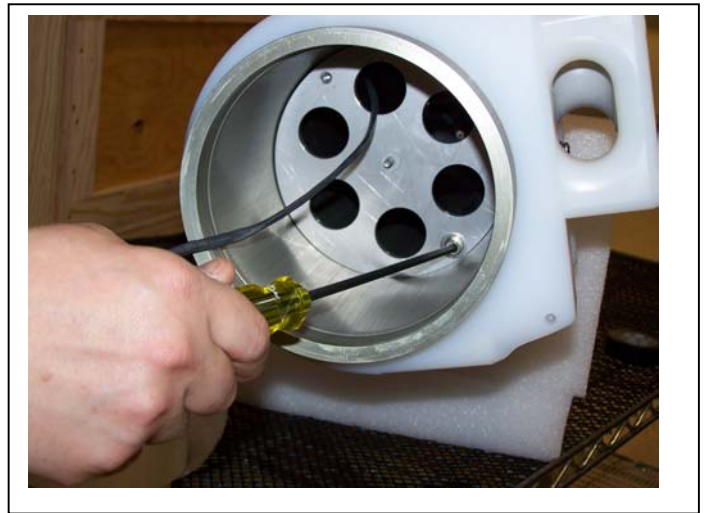
Figure 2-13: Secure Top Connecting Plate
