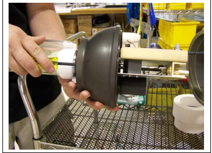
Figure F-13: Tighten Cap into Stud
