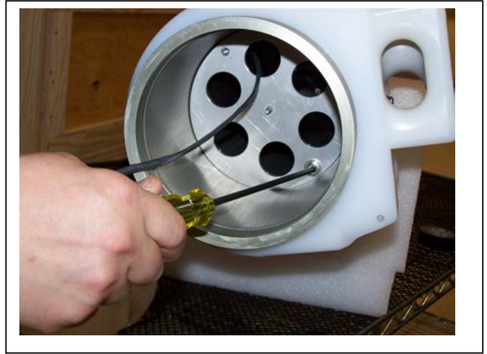
Figure F-9: Secure Top Connecting Plate
