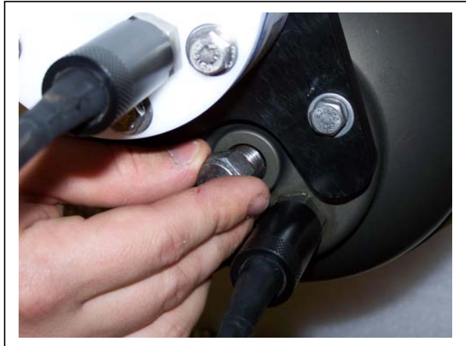
Figure 6-8: Remove the Bottom Plug
