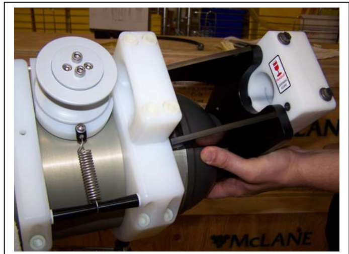
Figure 2-21: Position Inductive Modem
