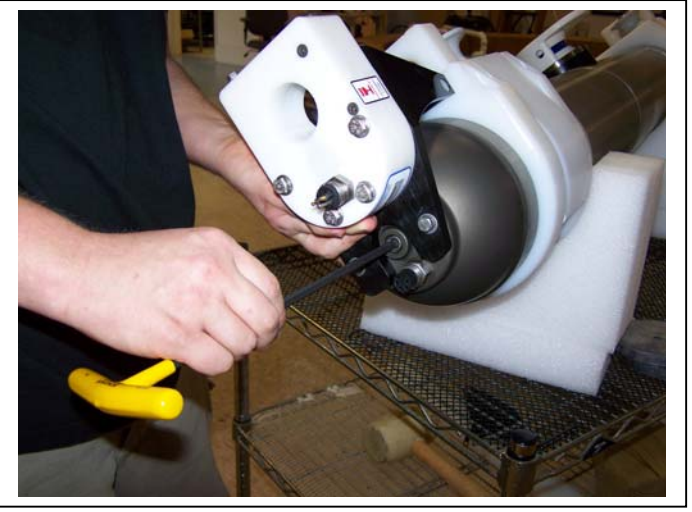
Figure 2-23: Tighten Socket Cap Screw
