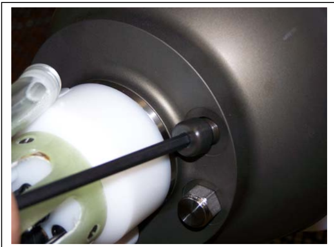
Figure F-14: Install Both Top Plugs
