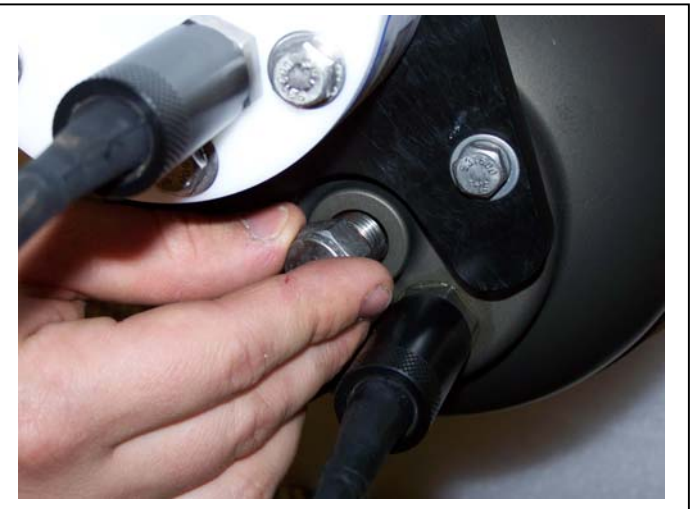
Figure 2-25: Install Bottom Plug
