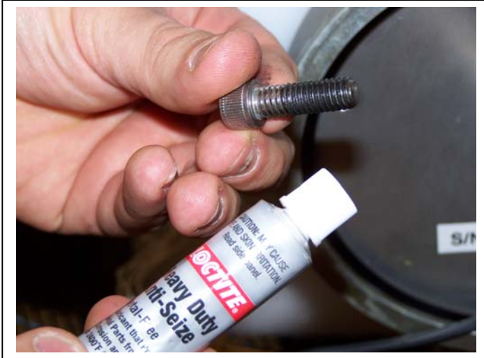
Figure 2-22: Apply Anti Seize Lubricant
