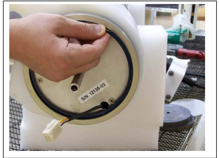
Figure F-7: Secure Retaining Ring
