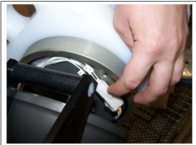
Figure 2-20: Coil UIM/COM Wiring Harness
