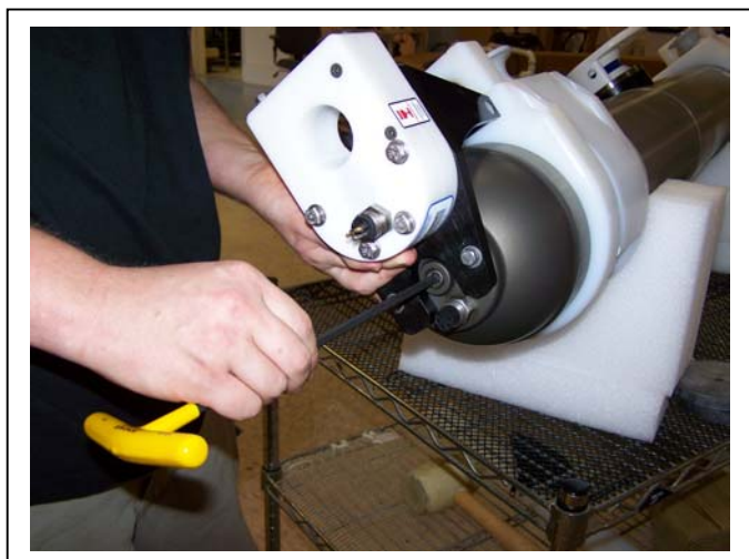
Figure 6-9: Loosen the Bottom End Cap Screw
