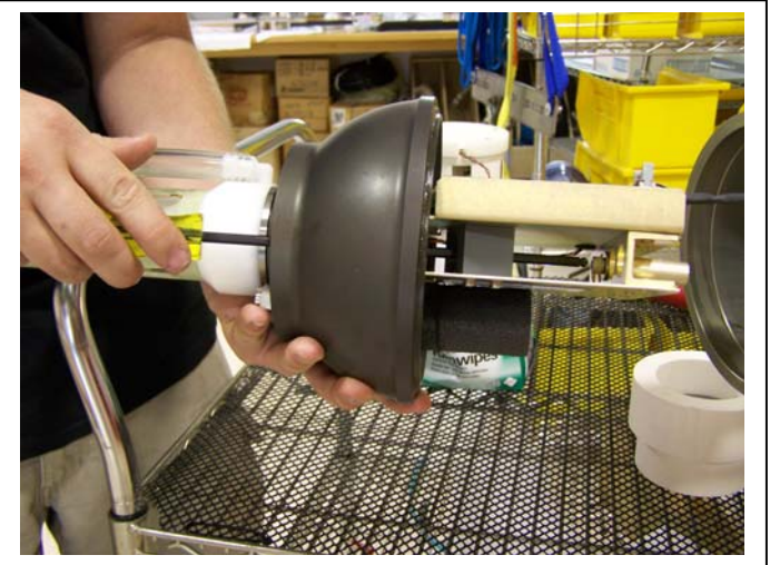
Figure 2-16: Tighten Cap into Stud
