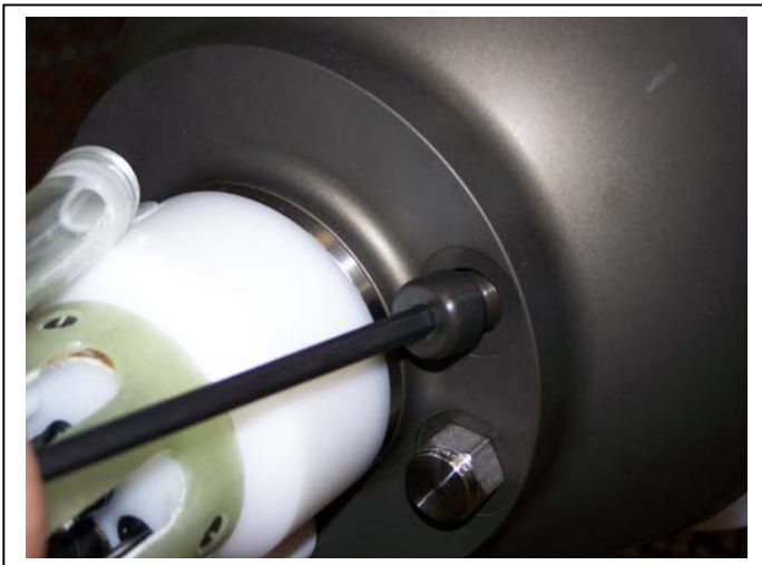
Figure 2-17: Install Both Top Plugs
