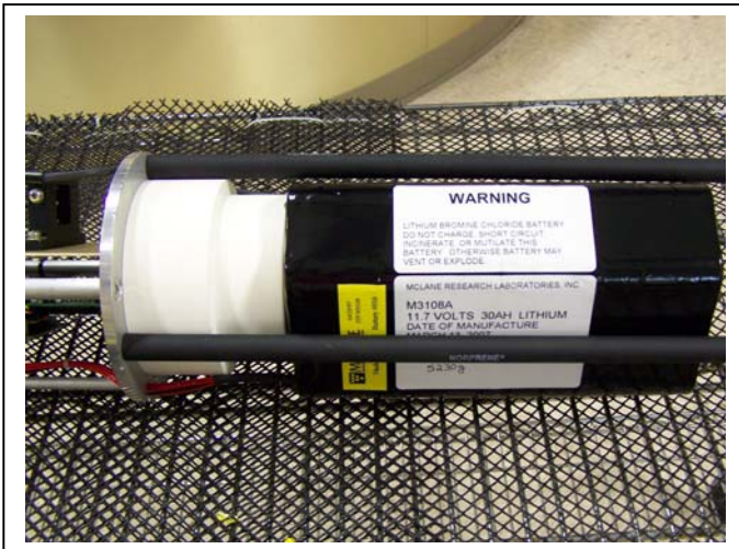
Figure 2-2: Battery Installed in Battery Holder
