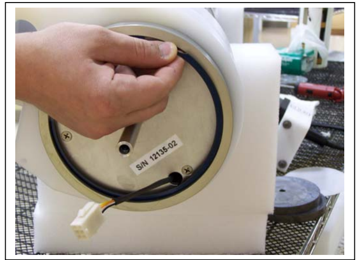
Figure 2-11: Secure Retaining Ring
