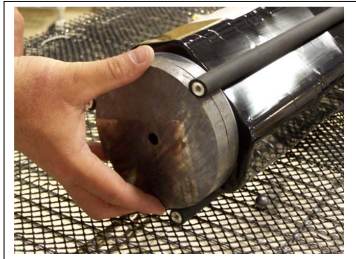
Figure 2-5: Lead Ballast Plates
