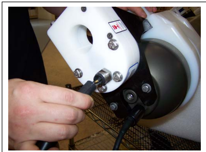
Figure 6-7: Disconnect the UIM Cable
