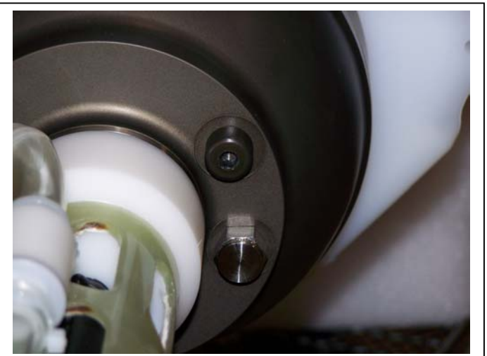
Figure 2-17: Install Both Top Plugs
