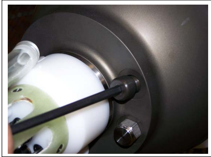
Figure 6-2: Remove CTD End Cap Plug
